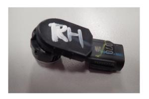
12. Using a paint pen or white marker, label each parking sensor (Left or Right) prior to removing from bumper.
