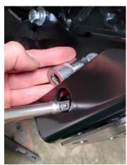
NOTE: IF USING A LARGE SIZE SOCKET, IT MAY BE NECESSARY TO PLACE THE SOCKET OVER THE FRONT BOLT BEFORE INSERTING AN EXTENSION THOUGH THE HOLE IN THE FLANGE.
