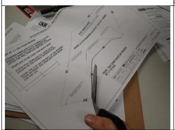
21. Carefully cut out bumper cut template supplied.
