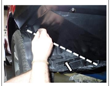
85. Mark lines onto the OEM inner guards (LH & RH) using lower edge of wing under panels as guide ensuring enough guard remains so that it may be neatly tucked/secured behind wing under panel lip.
