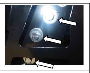
69. Loosely fasten bar to mounts using 6 x M12 x 1.75x35mm bolts, 6 x M12 flat washers (4mm thick) and 6 X M12 flange nuts.
