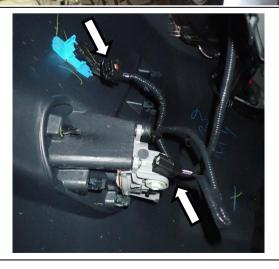
10. If equipped, disconnect fog light wiring and front parking sensors – (Right Hand side shown).
