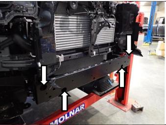
15. Remove 2 x M10 bolts on both sides (4 total) fixing crash beam to chassis and remove crash beam.
