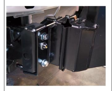
central to body, then tighten all fasteners joining mount assembly to chassis brackets (4x M10 and 2x M10 OE bolts each side).
