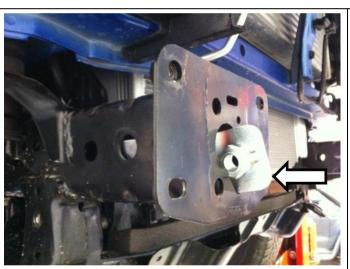
34. Insert 2 x M12x1.75 nut plates into RHS chassis rail as shown.
