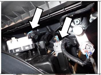
19. From the inside of the engine bay, unclip both the black and grey connectors from each headlight.
