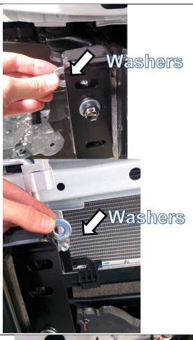
39. On both RH and LH installation it is extremely important that 1 x M10 x 25 x 3mm flat washer per hole is installed on the upper holes between the support brackets and the mount when offering the mount up to the chassis flange. The upper M10 bolts as installed in step below should pass through the mount, spacer washers and the support brackets.
