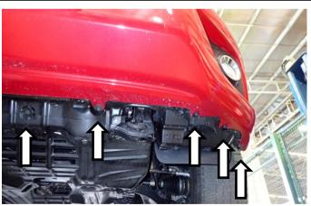
6. Remove all fasteners and scrivets retaining bumper along lower lip – (Left Hand side shown).
