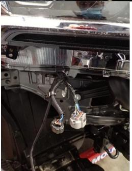
20. Following fitting instructions 3789197 supplied in kit 6821287; attach the LED combination lamp looms (also supplied in same kit). Vehicle coloured wires can be found in the positions indicated.
