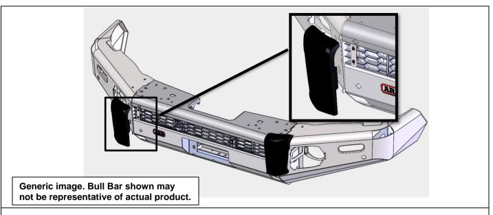
57. Ensure each buffer sits flat against the face of bar. Secure wing side using retaining clips. Secure inner side using the angled cup washers, flat washers and screws.
