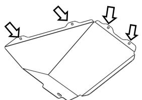
82. Fit 4 x M6 cage nuts to each wing under panel.
