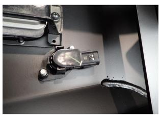
66. Fasten assembly to bullbar by torqueing M6 Nyloc nuts to specification.
