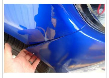
11. Remove registration plate and set aside, then carefully remove bumper from vehicle by pulling on each side of the bumper near the wheel arches and working your way towards the centre.
