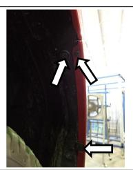
5. Remove all fasteners and scrivets retaining bumper along inside edge of wheel arches – (Right hand side shown).
