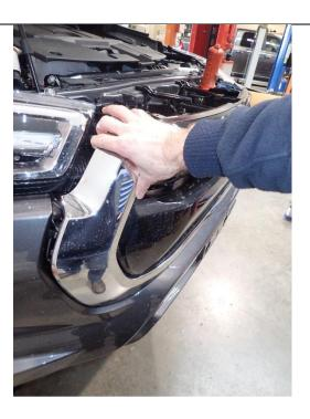
4. Gently unclip and pull back the top outside corners of the grille to reveal final two screws retaining grille. Using an extension and socket, remove and set aside for re-fitment later on.
