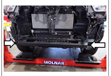
14. Remove plastic lower impact absorber from vehicle and discard.
