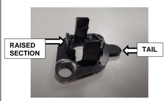
64. Assemble the sensor retaining plate onto the plastic retainer (set aside in step 13) so that the tail of the plate is on the opposite side to the raised section.
