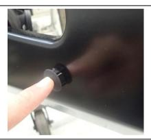
63. Press dome plugs into sensor holes in bar. (these will be used to accurately locate the sensor retaining brackets)
