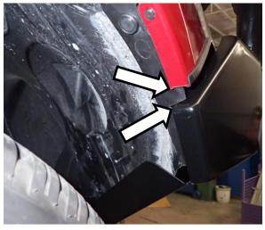
87. In line with the bottom edge of the lower bumper trim and the top edge of the bulbar wing tip use a pair of shears to cut a section approximately 20mm x 20mm from the inner guard outer edge to allow it to be pushed into the end of the wing. (RH Shown).
