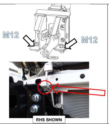
43. Loosely install 2 x M12 x 35 bolts and flat washers through lower mount and chassis support brackets into M12 flange nuts.
