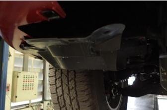
9. Ensure inner guards are unclipped from front bumper.
