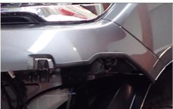
33. Fit Pinch weld to RH side along the full length of the cut edge. Carefully trim off any excess length and use remainder for other side.
