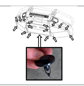
84. Fasten stone tray using 4x M8 bolts, flat washers and 2x M6 OEM fasteners
