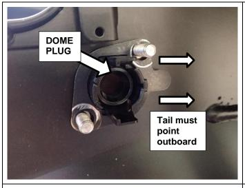
65. Assemble retainer and plate onto the inside of wing aligning mounting holes with studs. (tail outboard)
