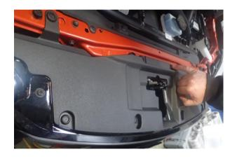
89. Re-install upper radiator cover panel and fasten using 8 x OE scrivets.
