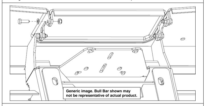
47. Fit the number plate bracket to the top face of the lower-centre pan on the bar using 3 x M6 x 20 hex bolts, flat washers and flange nuts.
