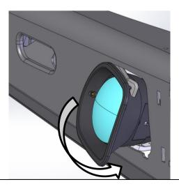
77. Assemble and install combination light surrounds (p/n 3163082) as per instruction no. 3789190 supplied with surround kit. Note: Optional LED fog lamps can be installed at this point as per fitting instruction supplied with fog lamp kit no. 3500910.
