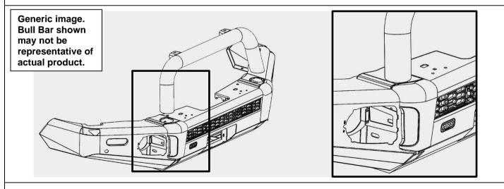
61. Fasten top tube to the bar using 4 x M10 SEMS Bolts. Adjust position of top tube left/right until it sits central on the bar and the rear buffers are positioned correctly. Tighten M10 SEMS Bolts to specification. Tighten Rear buffer screws.
