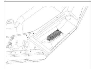
62. Fit the small square plastic grommets to the bar and attach the combination LED lamps to the bar using the screws provided with the lamp kit.
