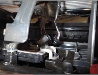
8. If vehicle is equipped with adaptive cruise control, unplug radar (located behind Toyota badge)
