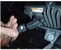
32. If vehicle is equipped with adaptive cruise control, reconnect radar.
