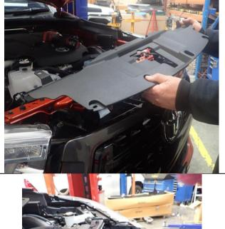
3. Remove upper grille retaining screws (4). Set aside for re-fitment later on.
