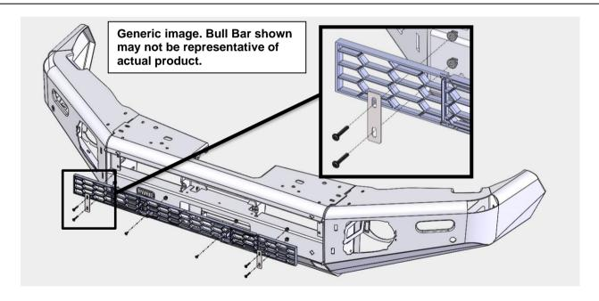
56. Place each of the front buffer sections onto the bar as shown. Ensure that the 2 lugs and 2 screw bosses pass through the holes in the bar.
