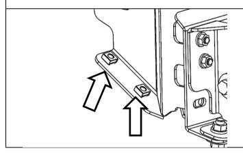
83. Fit 4x M8 cage nuts to RH and LH bull bar mounts as indicated. (RH Mount Shown)
