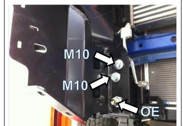
NOTE: MOUNTS ARE HANDED. RIPPLES ARE ON THE OUTSIDE OF MOUNTS
